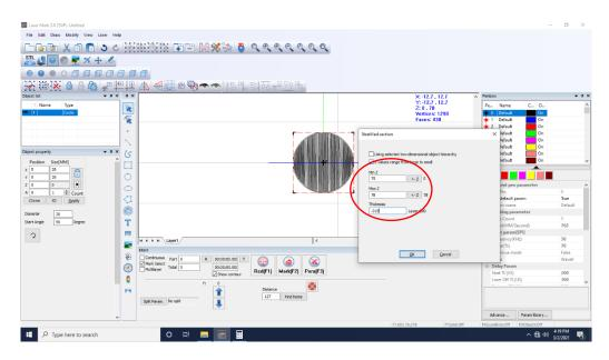
8. Click the "Add Contour" button to combine the slice and circle outline for removal of material outside of the STL. Place the cursor over the outside shape—when the cursor becomes a hand, click to create one sliced entity (skip if engraving the STL shape into the material instead of relieving material to reveal the shape)
