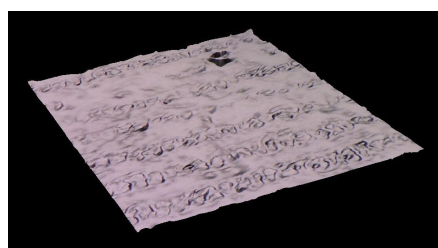
LC-53 (Level 1) Ra= 1.2 \mu\text{m}
