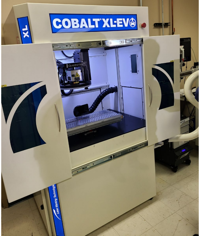
Cobalt-xl-ev-100PF laser making system 100-watt HO Ytterbium pulsed fiber LMT MOPA
