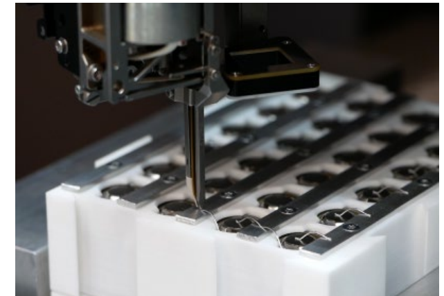
Wire Bonding process of Battery Pack [3]
