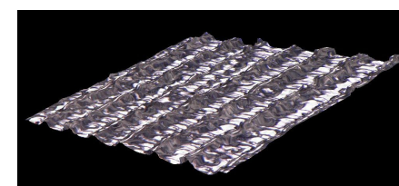
LC-46 (Level 3) Ra= 3.4 \mu\text{m}
