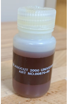
Blasocut 2000 Universal Cutting fluid based on Mineral Oil
