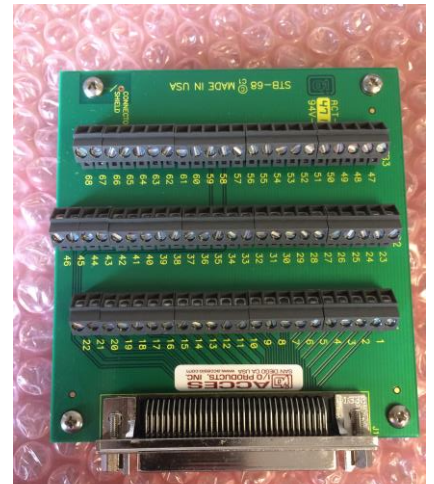
Pic1: Example photo of the green breakout board found in the lower right section of the electrical panel
