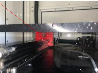
5. Using the software, run the Y table back in forth the length of the screw to work in the grease
